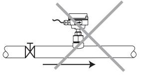
Post-valve cavitation can create air pocket
