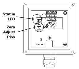
To perform the adjustment, after determining that there is a full pipe with no flow, short between the two pins marked "Zero Adjust". A red LED light will come on for approximately 50 seconds and then go out. The zero adjustment is completed.
