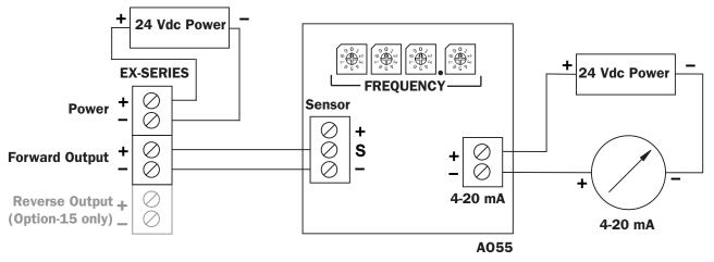
\*See Dual FT420 Diagram for an example of bidirectional connections.
