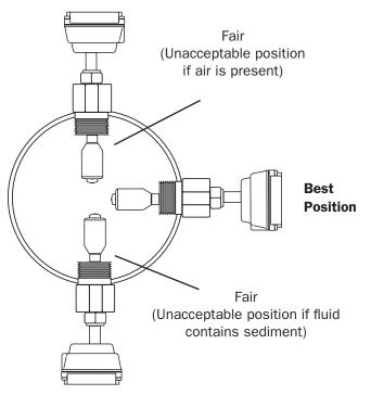
Horizontal is the preferred installation orientation, since it improves low-flow performance and avoids problems with trapped air and sediment. Bottom, top, and vertical pipe installations are all acceptable if required by the piping layout.
