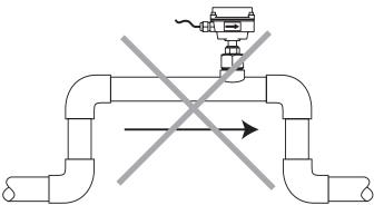
Allows air pockets to form at sensor
